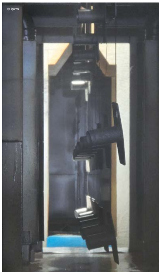
From left to right: The components undergo Chemtec's innovative TORAN 3 ® pre-treatment through a spray application process; The TORAN 3 ® pre-treatment is an anhydrous single-stage cold process; Components are coated with industrial polyester powders inside a Gema booth equipped with automatic spray guns.
