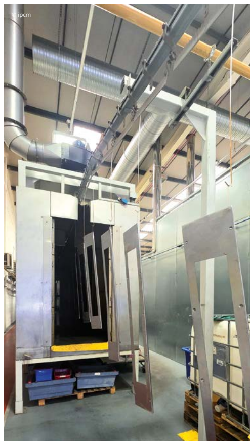
From left to right: The components undergo Chemtec's innovative TORAN 3 ® pre-treatment through a spray application process; The TORAN 3 ® pre-treatment is an anhydrous single-stage cold process; Components are coated with industrial polyester powders inside a Gema booth equipped with automatic spray guns.
