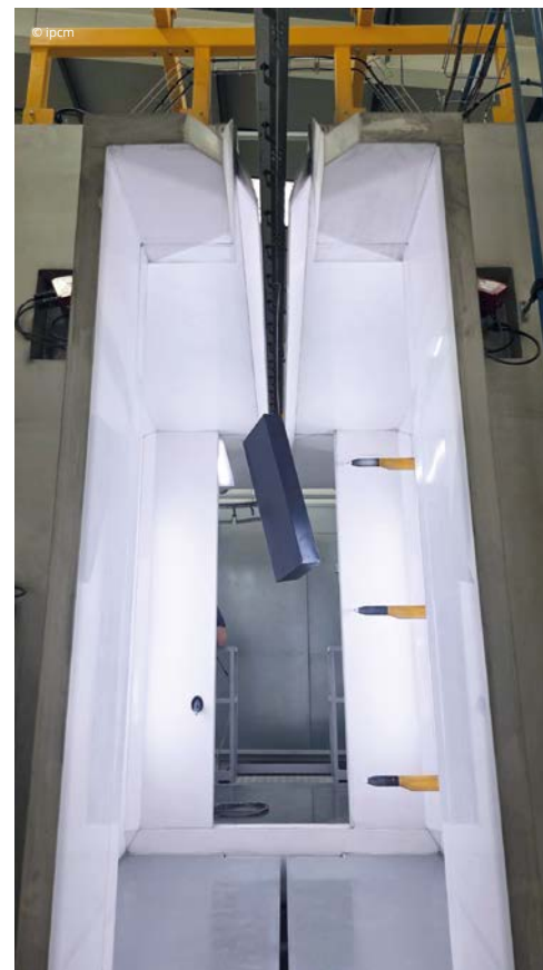
From left to right: The components undergo Chemtec's innovative TORAN 3 ® pre-treatment through a spray application process; The TORAN 3 ® pre-treatment is an anhydrous single-stage cold process; Components are coated with industrial polyester powders inside a Gema booth equipped with automatic spray guns.
